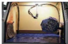
Fixing blasting head with rotating basket
